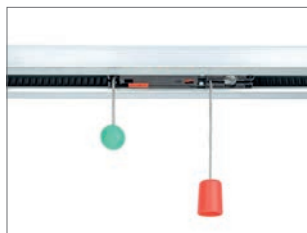
Emergency release The emergency release allows you to safely open and close your door in the event of a power cut. Pulling on the release will make the door disconnect from the opener, after which it can be manually operated.
