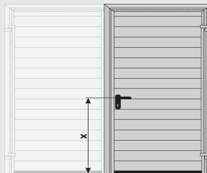
The section height and the height of the handle 'x' depend on the actual door height and construction of the door.
